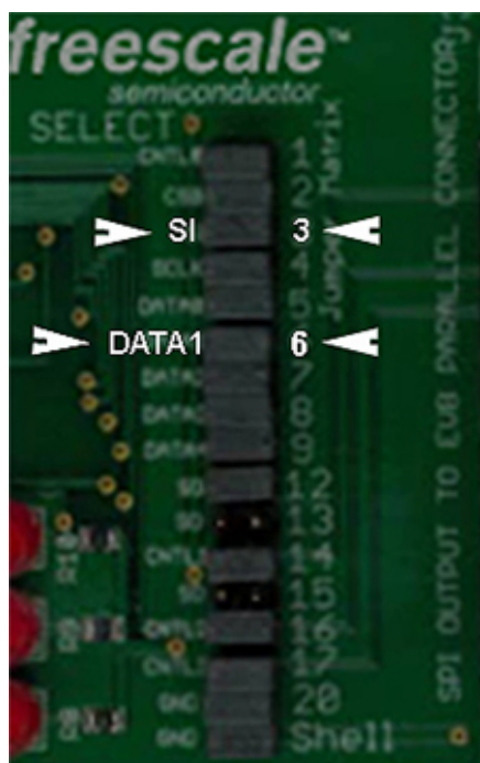
Figure 4. KITUSBSPIEVM Converter Board Jumper Matrix
