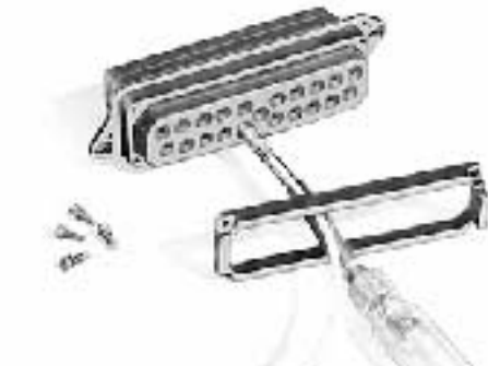
Inserting Coaxial & #12 Contacts
