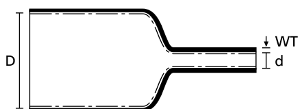
Heat Shrinkable Tubing 6:1 with adhesive
