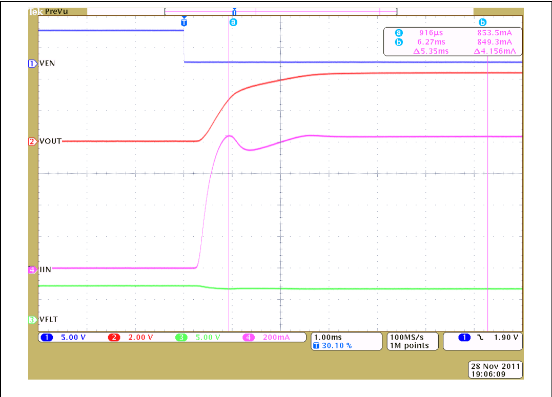
Figure 17. Soft-start performance for 100 \mu F capacitive load
