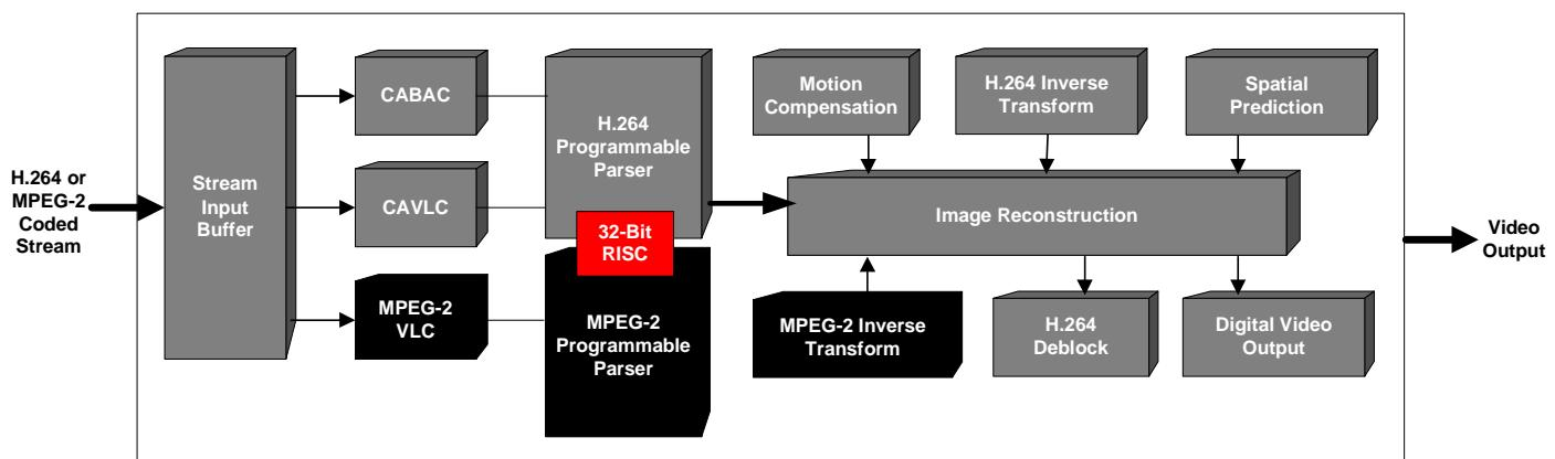
The BCM7411 introduces the advantages of the H.264 video compression algorithm to today's advanced consumer and broadcast applications. The BCM7411 is a dual-channel AVC/MPEG-2 decoder chip capable of full HD real-time decoding.
