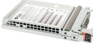
Streamlined installation and management, unrivaled scalability, and industry-leading virtualization support make the Emulex LPem11002-S dual-channel ExpressModule HBA an ideal solution for Sun Blade 8000 Modular Systems being deployed in storage area network (SAN) environments. The ExpressModule form factor provides a standardized method of deploying granular remote I/O that allows installation and removal of the Fibre Channel host bus adapter (HBA) without tools.
