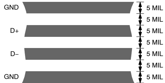
Figure 34. Typical Arrangement of Signal Tracks
