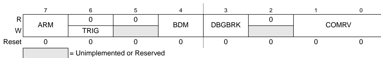
Figure 6-3. Debug Control Register (DBG1)
