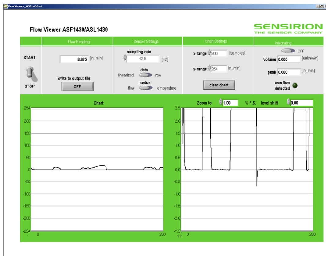
Figure 7: FlowViewer displaying measurement data of the EM_V (200 ln/min)
