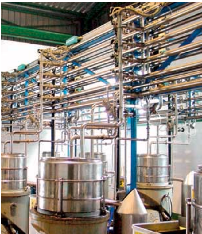
Control of the numerous valves using AS-Interface
