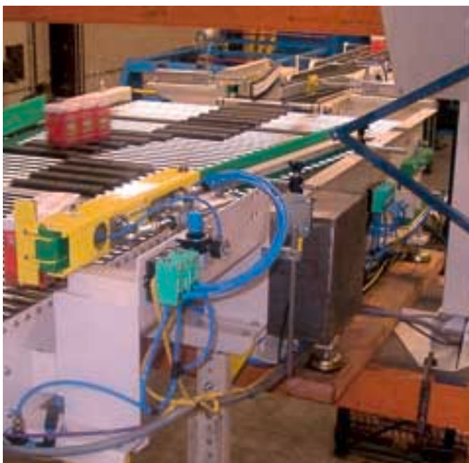
Conveyor system with pneumatic stoppers at the sorting point
