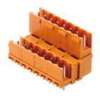
Dimensionally stable, straight, codable 2-tier male connector from the Unimate range of plugs with integral aid to prevent wrong connections. Available with open or closed sides. Fixing blocks can be attached to the closed version. The solder pin length of 3.2 mm has been optimised for wave soldering. Supplied in cardboard box.
