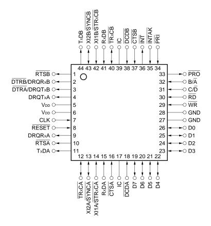
IC: Internally Connected (Leave this pin unconnected)
