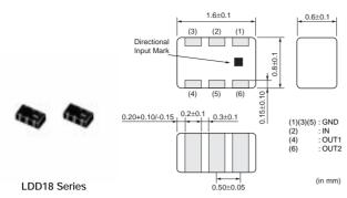
$100\Omega$  external resister is required between OUT1 and OUT2 All the technical data and information contained herein are subject to change without prior notice.
