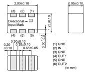
100ohm external resister is required between Out 1 and Out 2.
