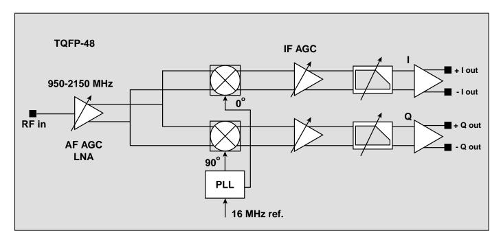
The **BCM3440** is a highly integrated CMOS tuner for the direct broadcast satellite (DBS) market. It is designed to operate with Broadcom's Advanced Modulation Receiver, the BCM4500, which supports 8PSK modulation with turbo code FEC. The **BCM3440** also operates with the BCM4201 QPSK satellite receiver. It is designed to support the full 1–45 Mbaud DVB operating range with support for 950 to 2150 MHz input frequencies.
