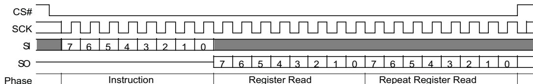
Figure 54. Read Bank Register (BRRD 16h) Command
