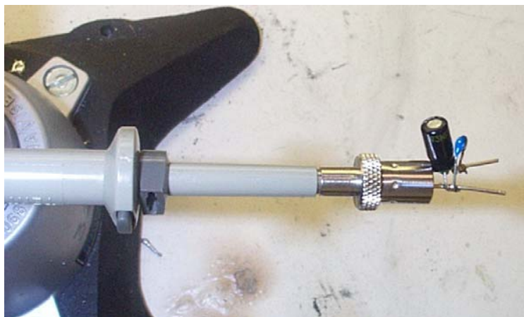
Figure 2 –Modified with wires for probe ground for ripple measurement, and two parallel decoupling capacitors added.
