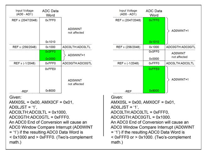
Figure 5.11. 12-Bit ADC0 Window Interrupt Example: Left Justified Differential Data
