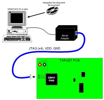
Figure 1.8. Development/In-System Debug Diagram
