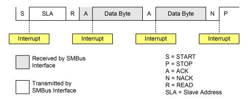
Figure 19.5. Typical Master Receiver Sequence
