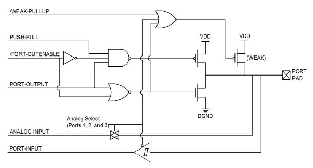
Figure 17.1. Port I/O Cell Block Diagram
