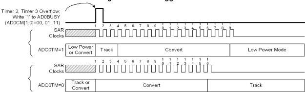
Figure 5.4. 12-Bit ADC Track and Conversion Example Timing
