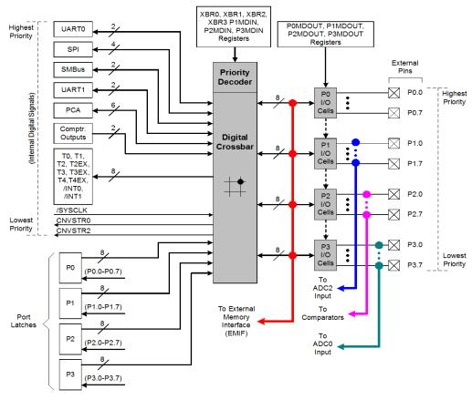
Figure 17.2. Port I/O Functional Block Diagram
