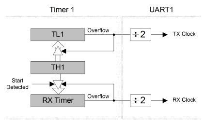
Figure 22.2. UART1 Baud Rate Logic
