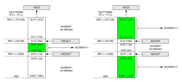
Figure 7.6. ADC Window Compare Examples, Differential Mode
