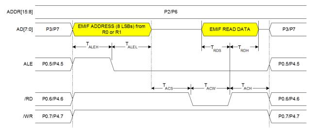
Figure 16.8. Multiplexed 8-bit MOVX without Bank Select Timing
