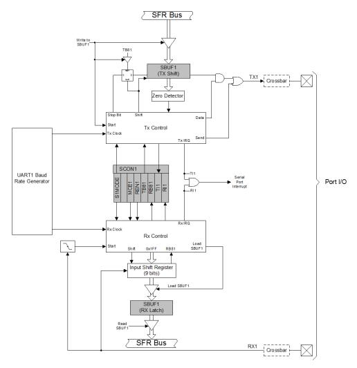
Figure 22.1. UART1 Block Diagram
