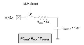
Figure 7.3. ADC2 Equivalent Input Circuit
