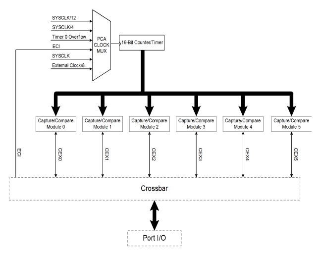
Figure 24.1. PCA Block Diagram
