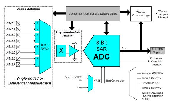
Figure 1.13. 8-Bit ADC Diagram
