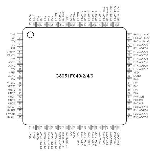
Figure 4.1. TQFP-100 Pinout Diagram
