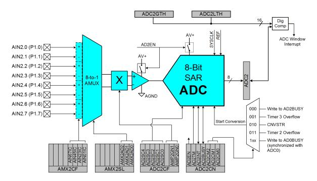
Figure 7.1. ADC2 Functional Block Diagram
