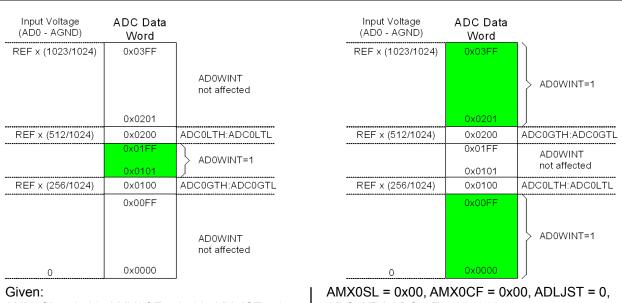
AMX0SL = 0x00, AMX0CF = 0x00, ADLJST = 0, ADC0LTH:ADC0LTL = 0x0200, ADC0GTH:ADC0GTL = 0x0100.
