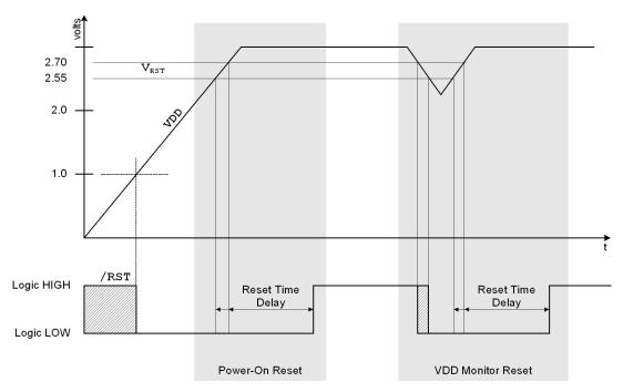
Figure 13.2. Reset Timing
