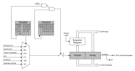
Figure 24.2. PCA Counter/Timer Block Diagram
