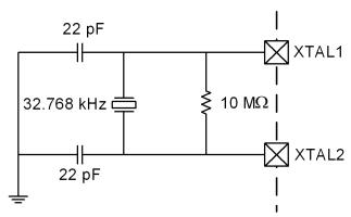
Figure 14.2. 32.768 kHz External Crystal Example
