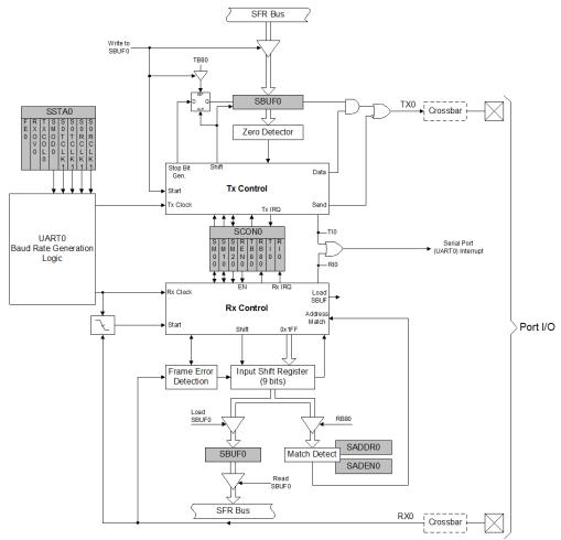
Figure 21.1. UARTO Block Diagram
