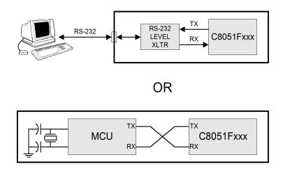
Figure 22.3. UART Interconnect Diagram
