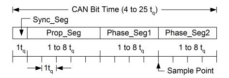
Figure 18.3. Four Segments of a CAN Bit Time
