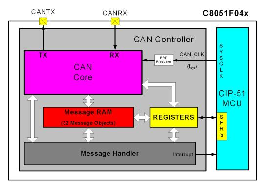
Figure 18.2. CAN Controller Diagram
