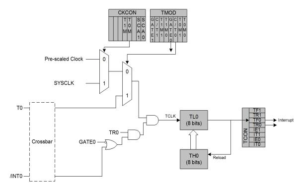
Figure 23.2. T0 Mode 2 Block Diagram
