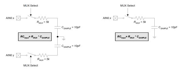
Figure 5.5. ADC0 Equivalent Input Circuits
