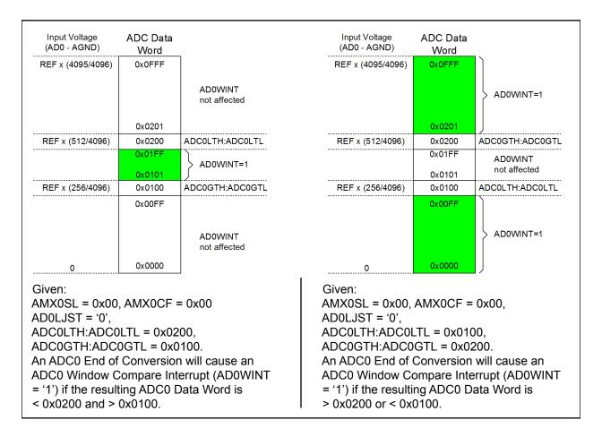
Figure 5.8. 12-Bit ADC0 Window Interrupt Example: Right Justified Single-Ended Data
