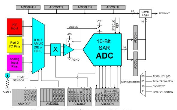
Figure 6.1. 10-Bit ADC0 Functional Block Diagram
