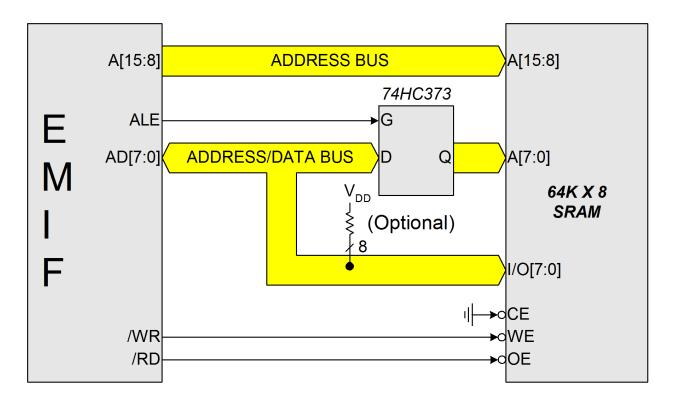
Figure 16.1. Multiplexed Configuration Example
