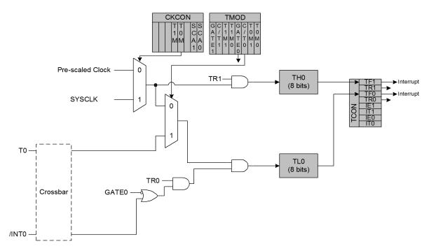
Figure 23.3. T0 Mode 3 Block Diagram
