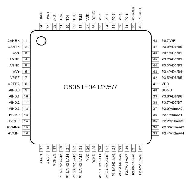
Figure 4.3. TQFP-64 Pinout Diagram
