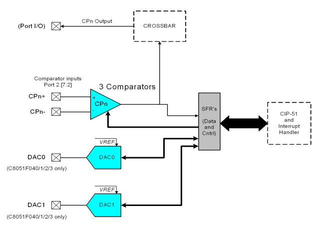
Figure 1.14. Comparator and DAC Diagram
