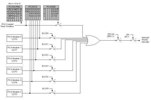
Figure 24.3. PCA Interrupt Block Diagram
