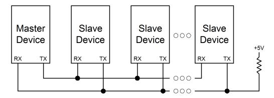
Figure 22.6. UART Multi-Processor Mode Interconnect Diagram
