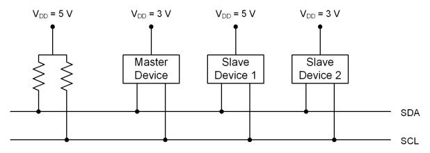
Figure 19.2. Typical SMBus Configuration
