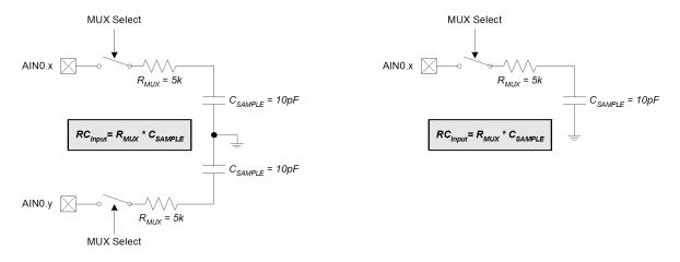
Figure 6.5. ADC0 Equivalent Input Circuits
