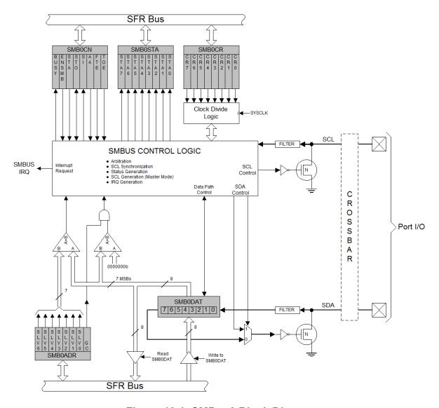
Figure 19.1. SMBus0 Block Diagram
