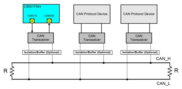
Figure 18.1. Typical CAN Bus Configuration
