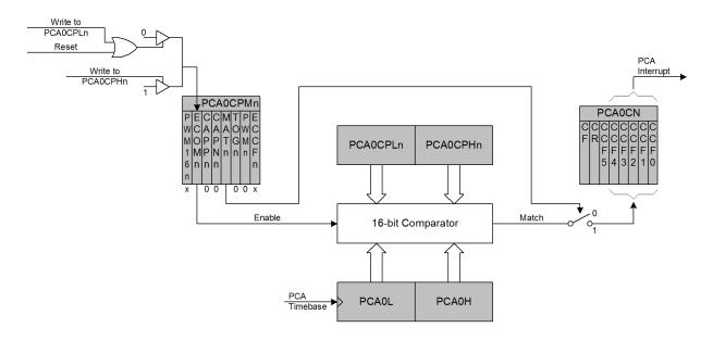
Figure 24.5. PCA Software Timer Mode Diagram
