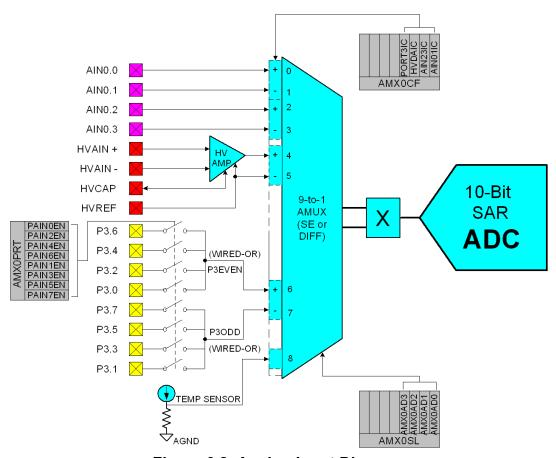
Figure 6.2. Analog Input Diagram
