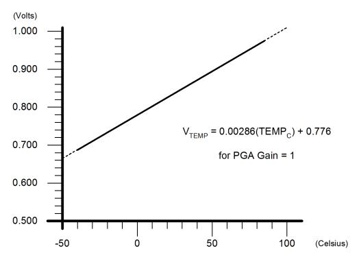
**Figure 6.6. Temperature Sensor Transfer Function**
