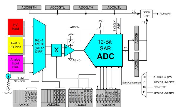
Figure 5.1. 12-Bit ADC0 Functional Block Diagram
