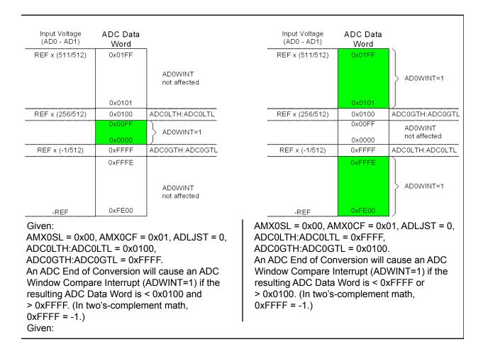
Figure 6.9. 10-Bit ADC0 Window Interrupt Example: Right Justified Differential Data
