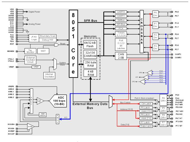
Figure 1.3. C8051F044/6 Block Diagram
