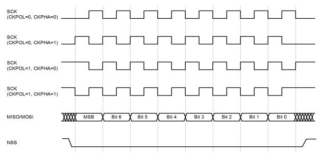
Figure 20.5. Data/Clock Timing Diagram
