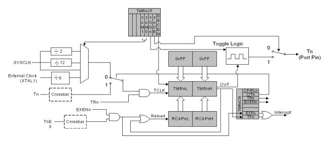
Figure 23.5. Tn Auto-reload Mode and Toggle Mode Block Diagram
