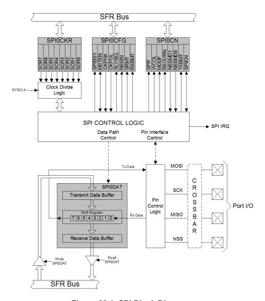
Figure 20.1. SPI Block Diagram
