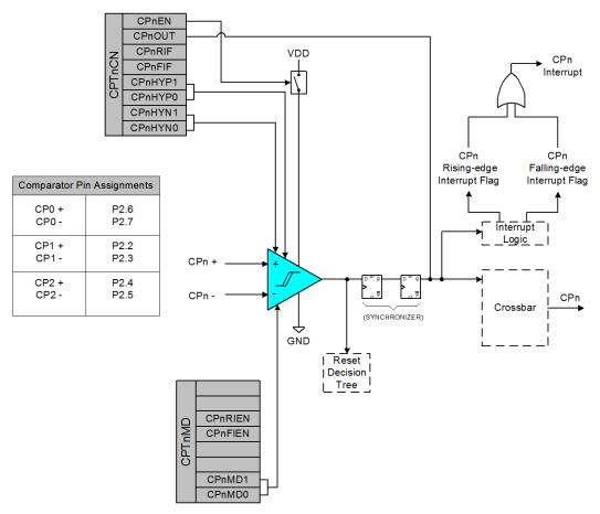
Figure 11.1. Comparator Functional Block Diagram
