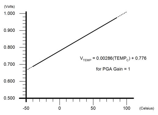
**Figure 5.6. Temperature Sensor Transfer Function**
