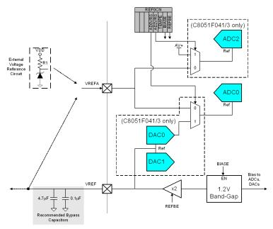
Figure 10.1. Voltage Reference Functional Block Diagram
