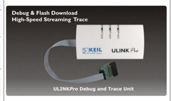
The Keil ULINK*Pro* Debug and Trace Unit connects your PC's USB port to your target system (via a JTAG, Cortex Debug, or Cortex Debug+ETM connector). It allows you to program, debug, and analyze trace information.
