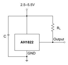
Notes: 4. C is for power stabilization and to strengthen the noise immunity, the recommended capacitance is  $10nF\sim100nF$ .  $R_L$  is the pull-up resistor, the recommended resistance is  $10K\Omega\sim100K\Omega$ .
