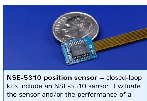
**NSE-5310 position sensor** – closed-loop kits include an NSE-5310 sensor. Evaluate the sensor and/or the performance of a closed-loop SQUIGGLE motor system.
