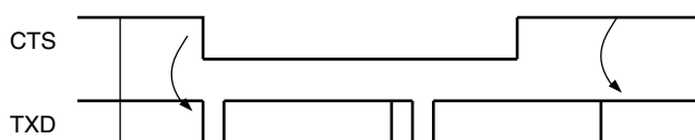
Figure 39-28. Transmitter Behavior when Operating with Hardware Handshaking
