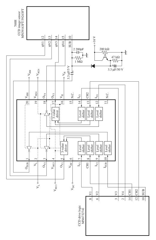
Note) Mount the bypass capacitors for the MN31121SA power supply pins (V<sub>HH</sub>, V<sub>H</sub>, V<sub>M13</sub>, V<sub>M24</sub>, V<sub>L</sub>, and V<sub>DC</sub>) as close as possible to the pin itself.
