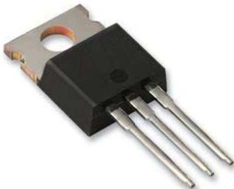
Fig. 1 Simplified Outline (TO-220C) and Symbol
