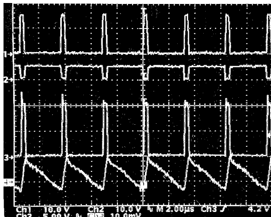
CH1: HDRV, CH2: LDRV, CH3: SW, CH4: I_L (0.2A/div) Output 1V @ 0.04A, V_{IN} = 10V, FPWM, L = 10 \mu H, f = 300kHz
