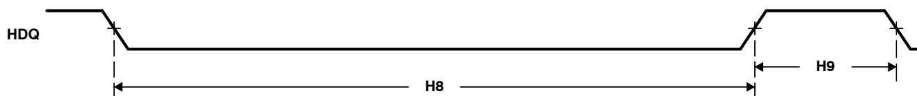
Figure 5–39. HDQ/1-Wire Break (Reset) Timing
