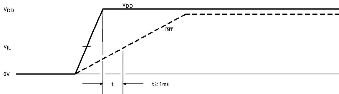
Adjust condenser value which is set  $\overline{INT}$  pin to the period while  $\overline{INT}$  pin is "L" level is longer than 1ms when power on.
