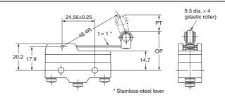
Note: Unless otherwise specified, a tolerance of  $\pm 0.4$  mm applies to all dimensions.
