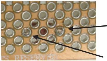
Touch the soldering iron to the SchmartSolder. You will see it quickly melt and fill the holes. Once you clip the excess component leads off, you will see very clean solder joints.
