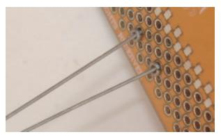
Put the SchmartSolder down to the base of the component leads .
