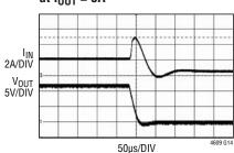
OUTPUT CAPS: 4x  $22\mu F$  CERAMIC CAPS AND 2x  $180\mu F$  ELECTROLYTIC CAPS 2x  $12m\Omega$  SENSING RESISTORS
