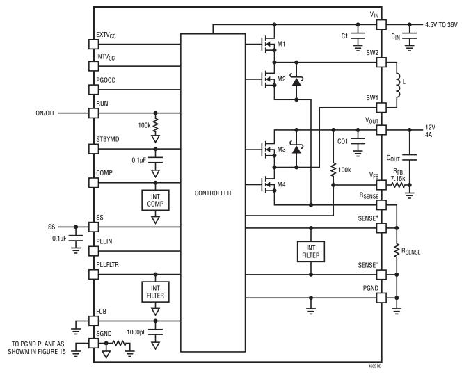
Figure 1. Simplified LTM4609 Block Diagram
