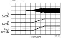
0.1 $\mu$ F SOFT-START CAP OUTPUT CAPS: 4x 22 $\mu$ F CERAMIC CAPS AND 2x 180 $\mu$ F ELECTROLYTIC CAPS 2x 12mΩ SENSING RESISTORS
