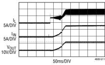
0.1µF SOFT-START CAP OUTPUT CAPS: 4x 22µF CERAMIC CAPS AND 2x 180µF ELECTROLYTIC CAPS 2x 12mΩ SENSING RESISTORS
