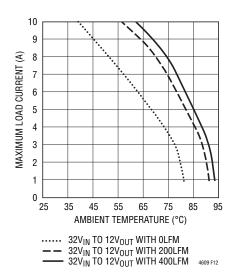
Figure 12. 32V<sub>IN</sub> to 12V<sub>OUT</sub> with Heat Sink
