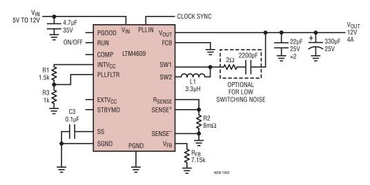
Figure 17. Boost Mode Operation with 5V to 12V Input with Low Switching Noise (Optional)
