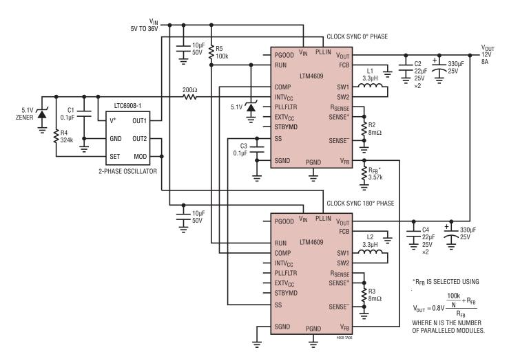
Figure 20. Two-Phase Parallel, 12V at 8A Design
