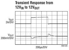
LOAD STEP: 0A TO 3A AT CCM OUTPUT CAPS: 4x 22µF CERAMIC CAPS AND 2x 180μF ELECTROLYTIC CAPS 2x 15mΩ SENSING RESISTORS
