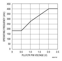
Figure 2. Frequency vs PLLFLTR Pin Voltage
