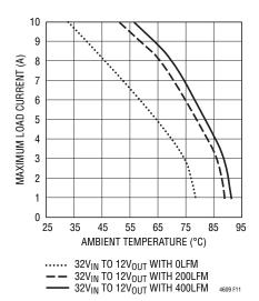
Figure 11. 32V<sub>IN</sub> to 12V<sub>OUT</sub> without Heat Sink
