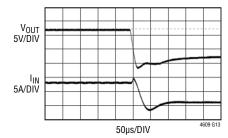
OUTPUT CAPS: 4x  $22\mu F$  CERAMIC CAPS AND 2x  $180\mu F$  ELECTROLYTIC CAPS 2x  $12m\Omega$  SENSING RESISTORS
