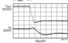
OUTPUT CAPS: 2x 10 $\mu$ F 50V CERAMIC CAPS AND 2x 47 $\mu$ F 50V ELECTROLYTIC CAPS 2x 15m $\Omega$  SENSING RESISTORS
