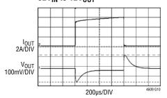
LOAD STEP: 0A TO 5A AT CCM OUTPUT CAPS: 4x 22μF CERAMIC CAPS AND 2x 180μF ELECTROLYTIC CAPS 2x 12mΩ SENSING RESISTORS
