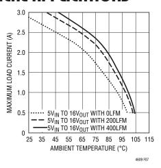
Figure 7. 5V<sub>IN</sub> to 16V<sub>OUT</sub> without Heat Sink
