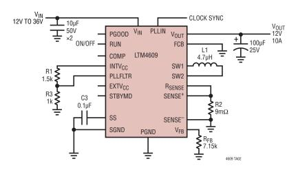
Figure 16. Buck Mode Operation with 12V to 36V Input
