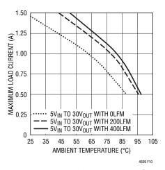
Figure 10.  $5\ensuremath{V_{IN}}$  to  $30\ensuremath{V_{OUT}}$  with Heat Sink
