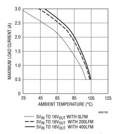
Figure 8. 5V<sub>IN</sub> to 16V<sub>OUT</sub> with Heat Sink
