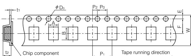
● Taping Reel Dimensions in mm (not to scale)
