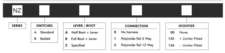
Polyimide tails only available with switch option A. Switch option A has pin terminals. Switch option B has solder terminals.
