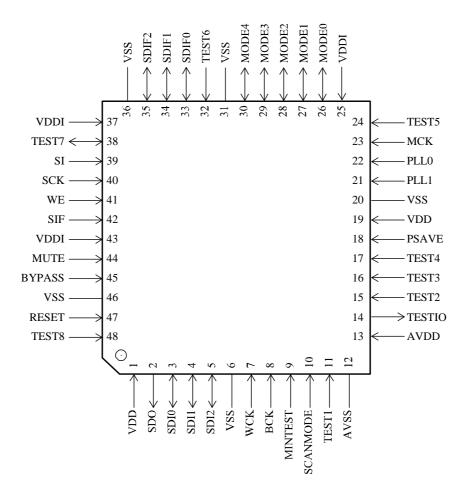
Note) All supply pins (VDD, VSS, VDDI, AVDD, AVSS) must be fixed. Connect MINTEST pin VSS.
