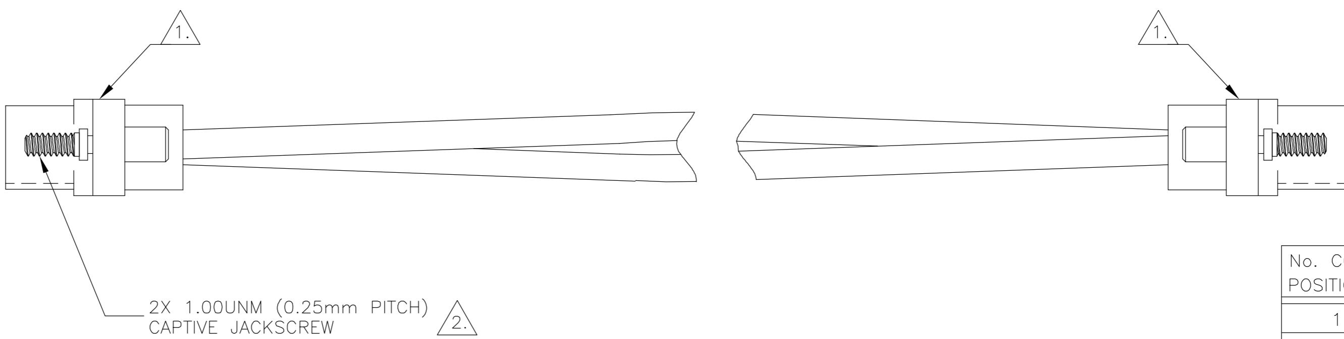
1. SHELL MATERIAL: 6061-T6 ALUMINUM, ELECTROLESS NICKEL PLATED PER SAE-AMS-C-26074
