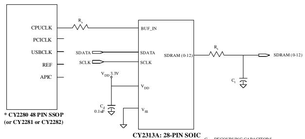
\* THIS FREQUENCY SYNTHESIZER IS USED TO GENERATE CPU, PCI, USB, REF, AND APIC CLOCKS.
