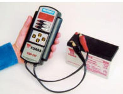
A new conductance tester from Yuasa Battery provides a simple method of checking the state of health of most 6V and 12V sealed lead acid batteries.
