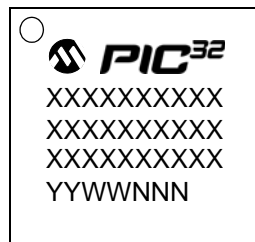
64-Lead QFN (9x9x0.9 mm)
