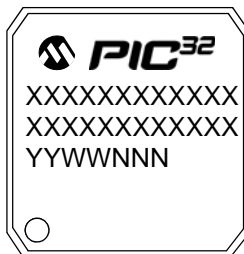
100-Lead TQFP (12x12x1 mm)
