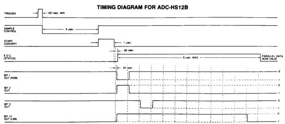
NOTE: TRIGGER, SAMPLE CONTROL, AND START CONVERT PULSES MUST BE EXTERNALLY GENERATED
