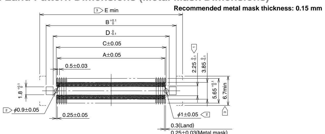
Note ① The cross-hatched area inside the SMT land may come into contact with the connector contacts and thus care should be taken that the pattern does not extend beyond the SMT land width.
