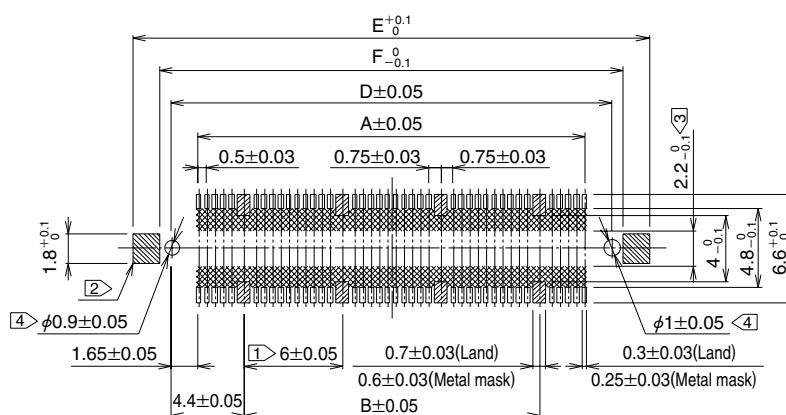
Note ① Cross-hatched portions, totaling n places, indicate the ground circuits.
