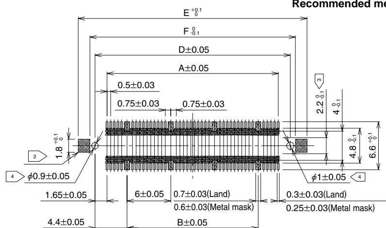
Note 1) Cross-hatched portions, totaling n places, indicate the ground circuits.
