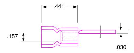
Max Electric Currrent: 22-16 AWG : 19 Amp Max Electric Rating: 75° C / 600 V Max
