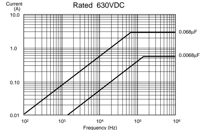
**Typical Characteristic Curves** Remarks : Typical curves are as shown below. (Slightly different depending on individual rating.)
