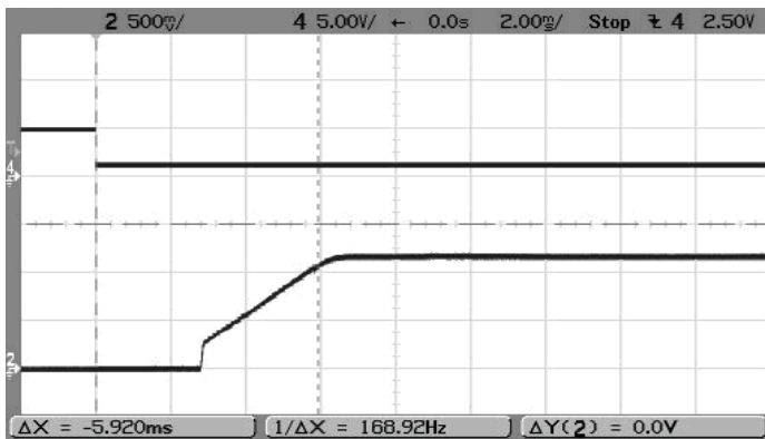
On/Off Enable Startup Delay (Vin=12V, Vout=1.2V, Iout=3A, Cload=0) Trace 4=Enable In, Trace2=Vout
