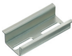
TS 35/15 mm according to EN 50022 (s = 1.5 mm)
