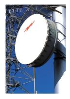
2.4 m | 8 ft High Performance Parabolic Shielded Antenna, single-polarized, 10.200–10.700 GHz, UBR100, gray antenna, enhanced white radome with flash, standard pack—two-piece reflector
