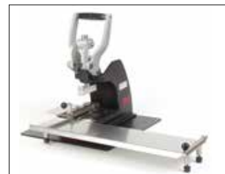
3M™ Standard Assembly Press, Model 3640 and 3M™ Locator Plate 3443-82-XX
