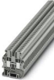
Mini feed-through terminal block, Connection method: Screw connection, Cross section: 0.2 mm<sup>2</sup> - 4 mm<sup>2</sup>, AWG: 24 - 12, Width: 5.2 mm, Color: gray, Mounting type: NS 15
