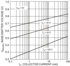
Fig. 6 Typical Base-Emitter Voltage vs. Collector Current
