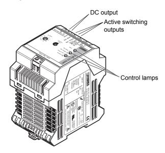
The connection is established through the "OUT DC 24 V, +, –" screw connections. The set output voltage is 24 V DC at the time of delivery. The output voltage from 22.5 V DC to 29.5 V DC can be set on the potentiometer.
