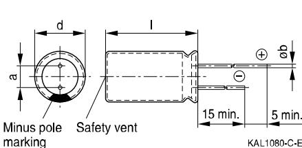
Safety vent for diameter  $\geq 6.3$  mm.
