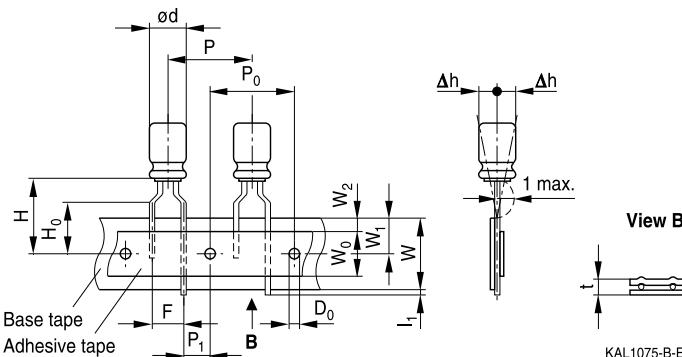
**Lead spacing 5.0 mm (from  $d \times l = 10 \times 12.5$  mm to  $12.5 \times 30$  mm)**
