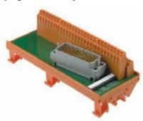
Weidmuller's passive interface units are used for adapting hermaphrodite ELCO multi-pole connectors, for input and output, to screw terminal systems. The hermaphrodite contact is a fork-type contact that is identical in design on both sides of the connection, but with one fork turned through 90° to engage with the other.
