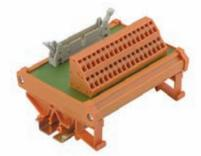
Passive interface for 10 ... 64 signals for adapting preassembled leads with plug connectors to IEC 603-1 / DIN 41651 to screw or tension clamp connection systems.
