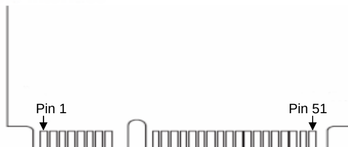
Figure 1-2 Apacer SDM M1 pin assignment
